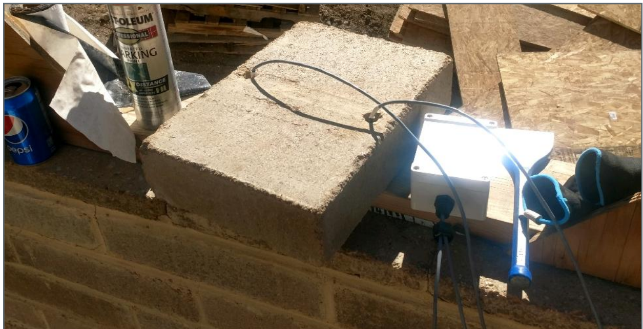
Image 15: A CEB block being prepared with the two embedded sensors.
