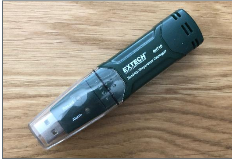
Image 10: Extech RHT10 data loggers used to record conditions in the Great Room as well as ambient conditions outside the building.
