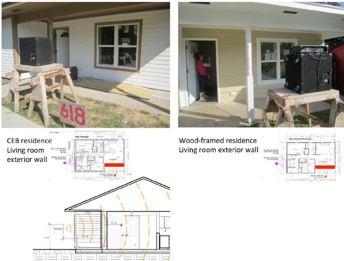
Figure 11: Images depict setting up sound source for north living room wall data collection in presentation slide format from ASA October 2014 meeting
