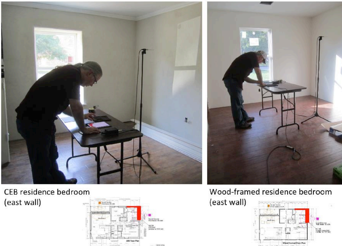
Figure 12: Recording NC and NIC values in presentation slide format from ASA October 2014 meeting. Images depict microphone placement of 5'-3" AFF and 3'-0" from interior surface.
